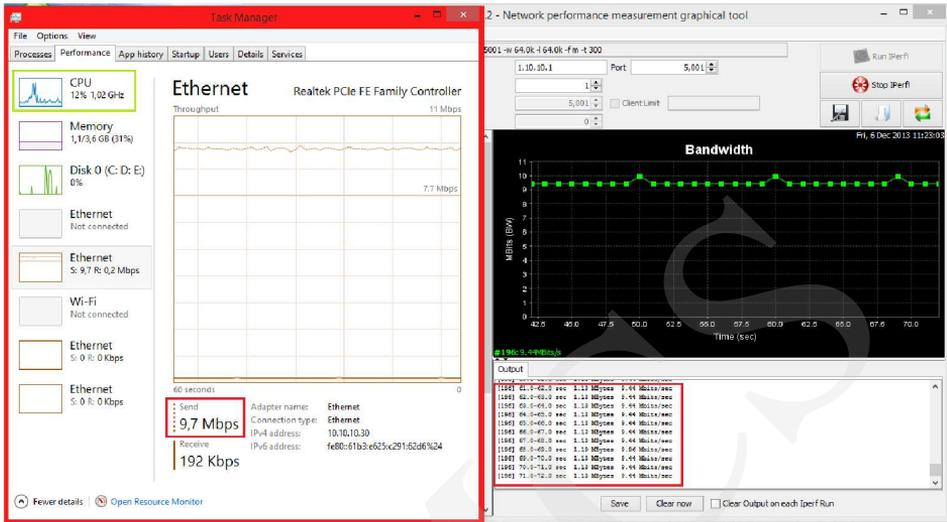
Fig. 5. 10Mbit/s link measurement without VPN tunnel.
