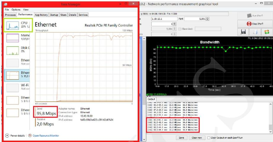
Fig. 3. 100Mbit/s link measurement without VPN tunnel.
