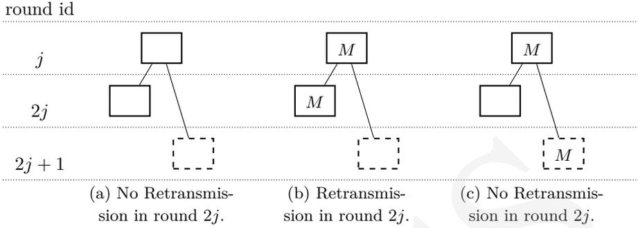
**RYSUNEK 3.** Collision resolution in SICTA. Only a message involved in a collision in round  $j$  may be retransmitted also in round  $2j$ . The round  $2j + 1$  is virtual; no transmission takes place. No new message can be sent until all collisions are resolved.
