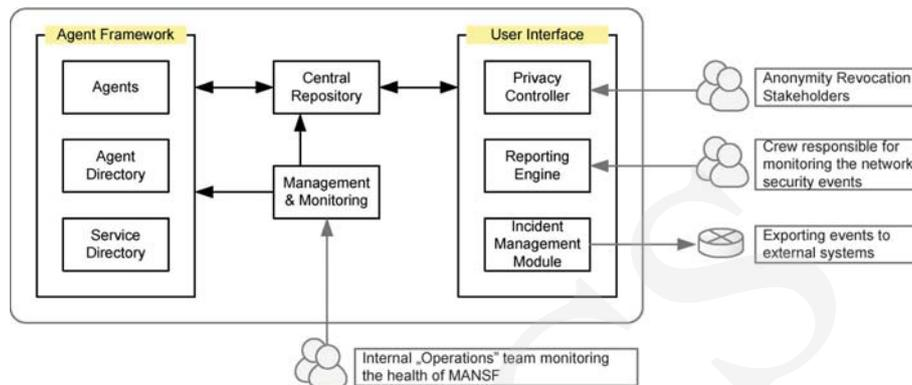
Fig. 1. Distributed network surveillance architecture.
