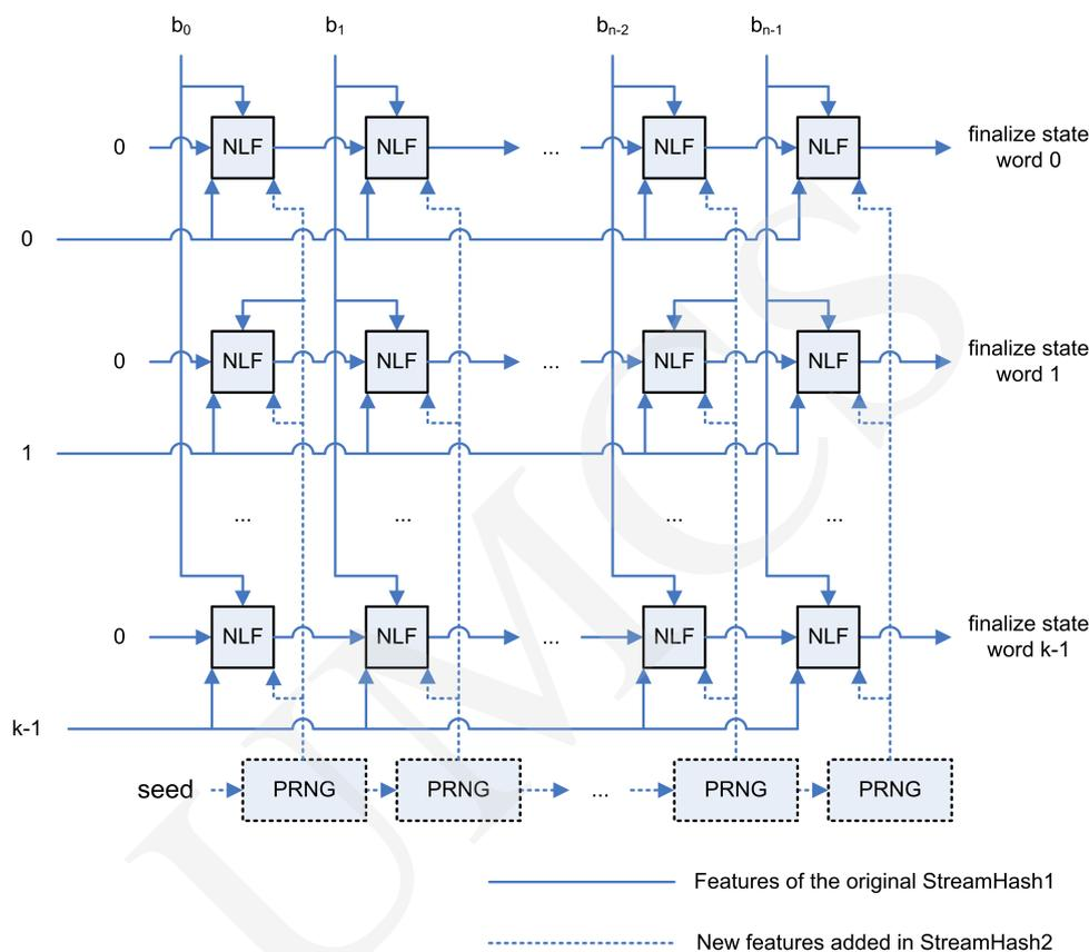
Fig. 2. StreamHash structure.
