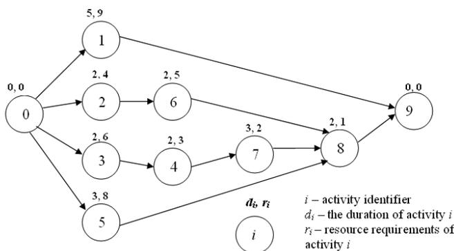
Fig. 1. Exemplary project network in the activity-on-node representation.
