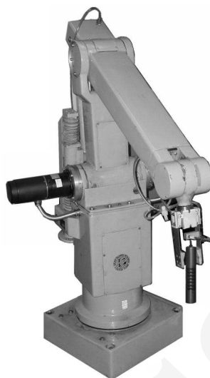
Fig. 1. 5-DOF robotic arm with the gamma radiation detector – the example of the use of the standard manipulator arm for manipulations in radioactive environments
