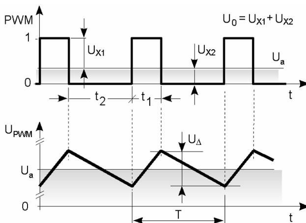
Fig.3. Saw-shape deformation of the analog PWM signal
