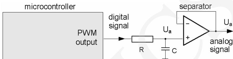
Fig. 1. Block diagram of the DAC\_PWM converter
