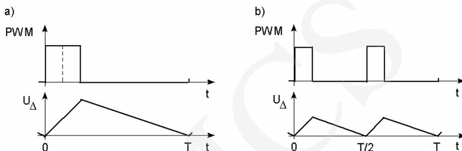
Fig. 4. Effect of digital PWM signal shape on the pulsation amplitude  $U_D$ :
